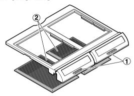
The Optibin Crispers provide fresher-tasting fruit and vegetables by letting you easily control humidity inside the crisper. The Optibin Crispers include: 1) a humidity control knob at the front of the crisper cover and 2) a large lattice on the inner surface of the cover to hold or release moisture.
